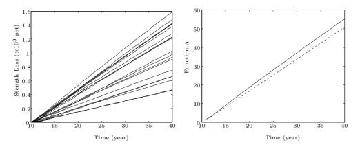
Figure 5.3. The left panel is the bridge beams' strength loss over time. The right panel is the estimated  $\tilde{\Lambda}_n$ , where the solid line is the maximum pseudo-likelihood estimator and the dashed line is the parametric estimator.
