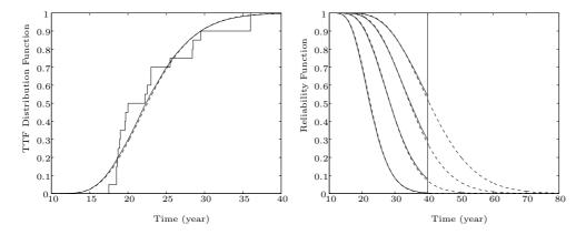
Figure 5.4. The left panel is the estimated time-to-failure distribution function of bridge beams for d = 400. The right panel is the reliability estimation for bridge beam at four different threshold levels, d = 400, 600, 800, 1000. The solid lines are maximum pseudo-likelihood estimators and the dashed lines are the parametric estimators.
