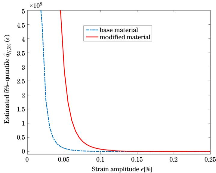
Figure 3. Comparison of the estimated 5%–quantiles of the number of cycles until the failure occurs  $\hat{q}_{N,5\%}$  from the base and the modified material of ZStE500. Here the strain amplitude is divided by the length of the material sample used in the experiments.
