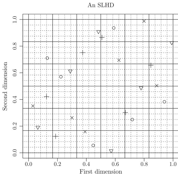
Figure 2. An SLHD based on the sliced Latin hypercube in Table 1. Points denoted by the same symbol consist of one slice of Latin hypercube design. For each dimension, each of the 24 equally spaced intervals of  $[0, 1)$  contains exactly one point and each of the six equally spaced intervals of  $[0, 1)$  contains exactly one point from each slice.
