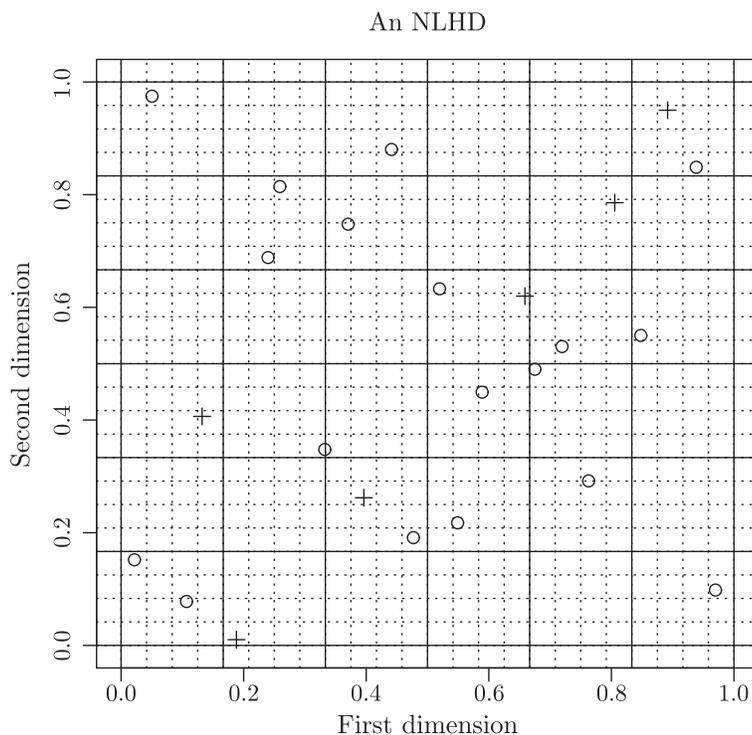
Figure 1. An NLHD based on the nested Latin hypercube in Table 1. The six points denoted by “+” consist of the nested smaller Latin hypercube design. For each dimension, each of the 24 equally spaced intervals of  $[0, 1)$  contains exactly one point and each of the six equally spaced intervals of  $[0, 1)$  contains exactly one point from the nested smaller design.
