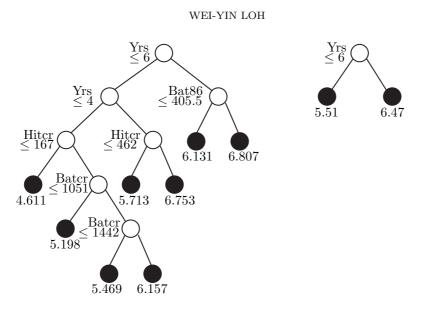
Figure 2. Piecewise constant (left) and piecewise linear (right) 1-SE GUIDE trees for baseball data with median split points. The piecewise constant 0-SE tree has 32 terminal nodes. The piecewise linear 0-SE and 1-SE trees are the same. The number beneath a node is the sample Y-mean.
