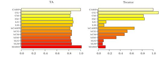
Figure 5. Barcharts of prediction mean square error relative to CART for the results in Table 11. CG and CM refer to the GUIDE piecewise constant tree methods with G and M split points, respectively, SM the piecewise simple linear method with M split point, and LG and LM the multiple linear methods with G and M split points. The b in a label indicates bagging. The bars are arranged in the same order as the rows of Table 11.
