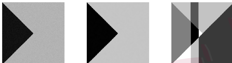
Figure 1: Demonstration of partitioning of the pixels in the test image. Images from left to right are the noisy image, the denoised image by the proposed method, and estimated partitions, respectively. The partitions are represented by different shades. Note that the estimated partitions are subsets of the true partitions.
