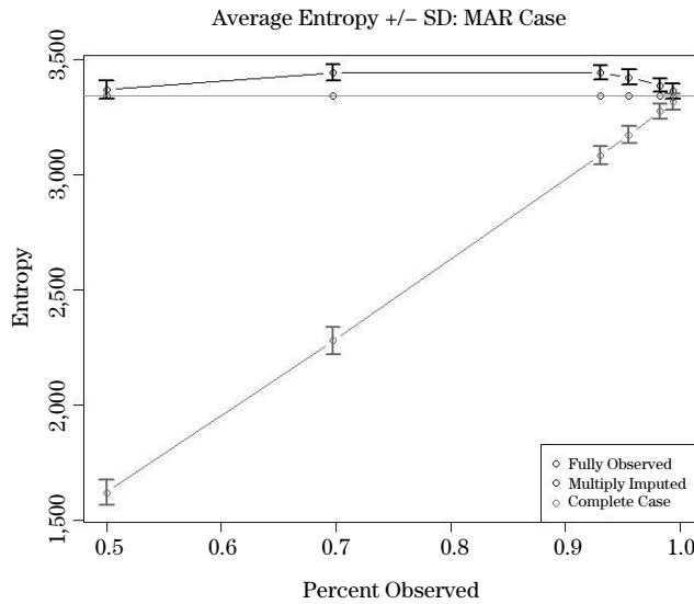
Figure 5. MAR case. Horizontal line: theoretical fully observed entropy. Center circles: estimated fully observed entropy. Dark grey: MI-based estimated entropy. Light grey: CCA estimated entropy. Bars:  $\pm$  one standard deviation.
