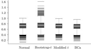
Figure 1. Boxplots of lower and upper confidence limits for the correlation coefficient based on 2000 simulated data sets from a double exponential regression family with correlation 0.5.
